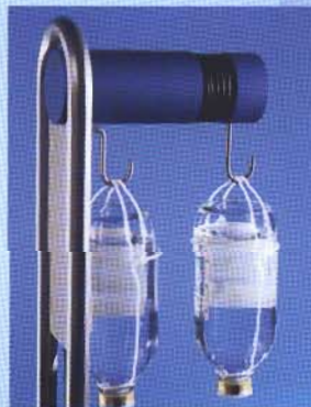
Volume transducer Attached firmly to the stand, designed to accommodate two infusion bottles
